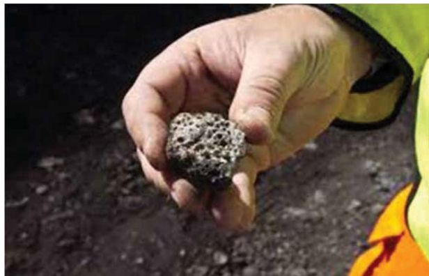
Figure 1. Example of tar bound material
