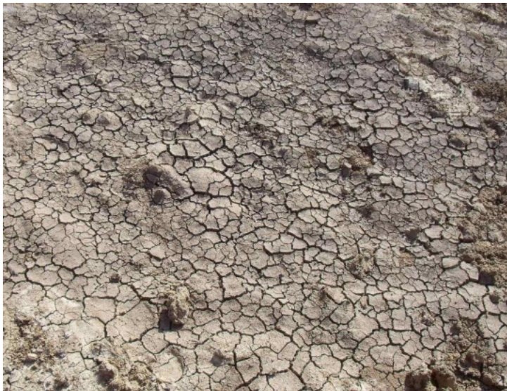
Plates 1: Desiccation cracks in a clayey sandy silt and an overconsolidated clay
