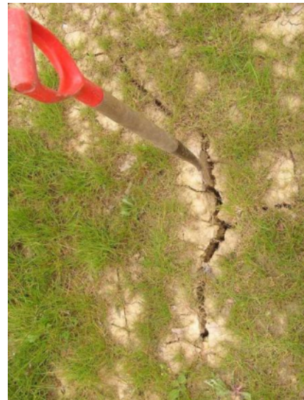
Plates 1: Desiccation cracks in a clayey sandy silt and an overconsolidated clay
